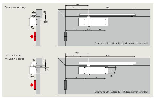
A 180° opening angle is possible in this installation type, provided that the appropriate construction conditions are met. In most cases, the door closer requires a wall recess for that purpose.
